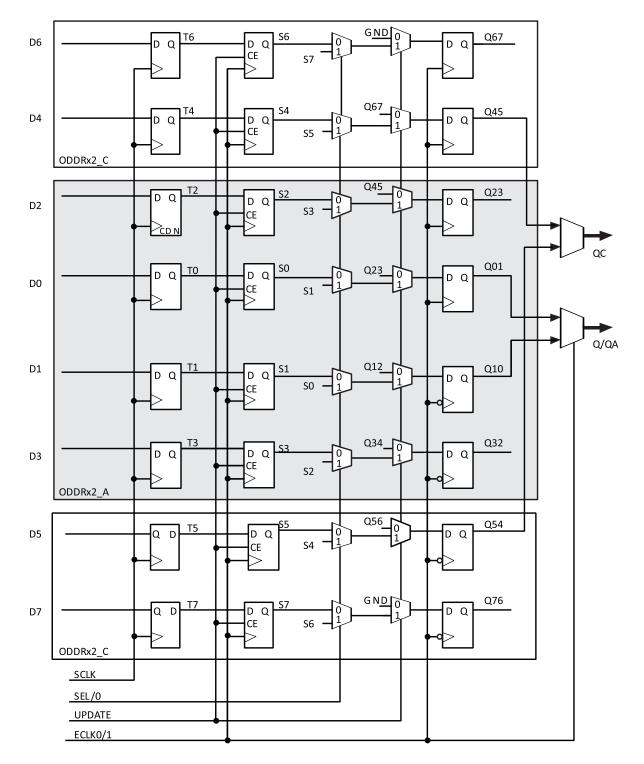
Figure 2.13. Output Gearbox
