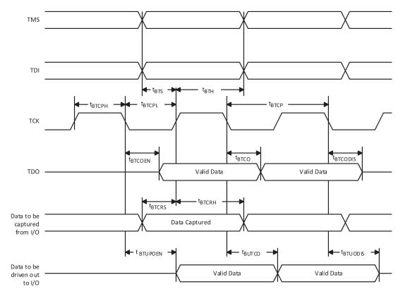
Figure 3.8. JTAG Port Timing Waveforms
