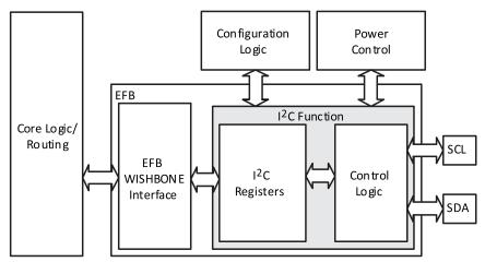
Figure 2.17. I<sup>2</sup>C Core Block Diagram
