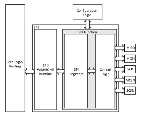
Figure 2.18. SPI Core Block Diagram
