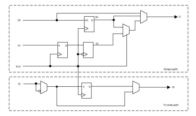
Figure 2.11. MachXO3D Output Register Block Diagram (PIO on the Left, Top and Bottom Edges)
