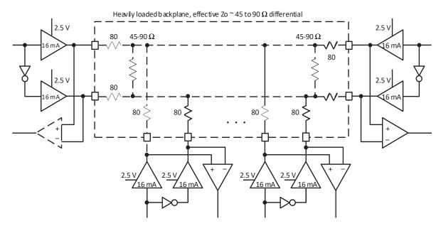
Figure 3.2. BLVDS Multi-point-Output Example
