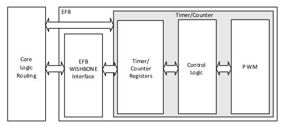
Figure 2.19. Timer/Counter Block Diagram
