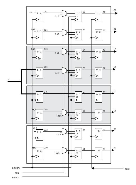
Figure 2.12. Input Gearbox
