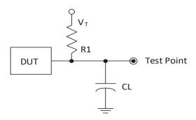
Figure 3.9. Output Test Load, LVTTL and LVCMOS Standards
