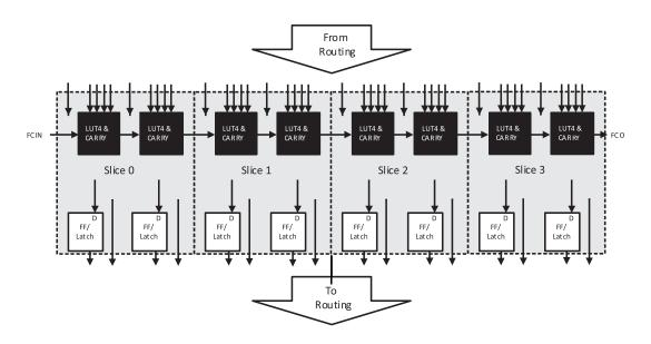
Figure 2.2. PFU Block Diagram
