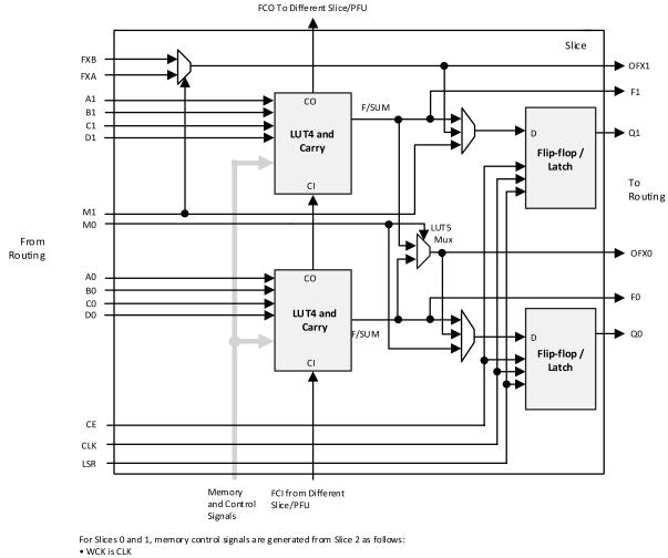
• WRE is from LSR • DI [3:2] for Slice 1 and DI [1:0] for Slice 0 data from Slice 2
