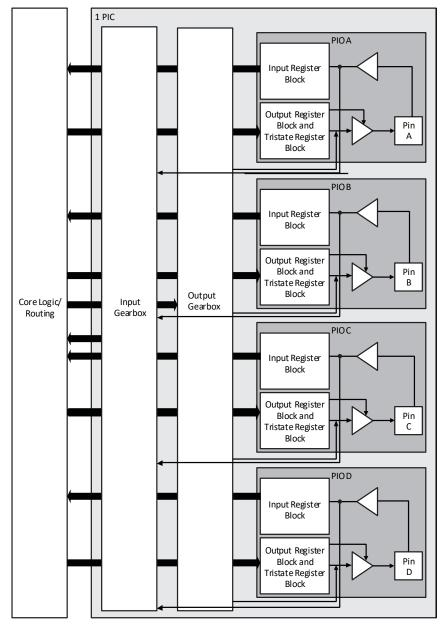
Figure 2.10. Group of Four Programmable I/O Cells
